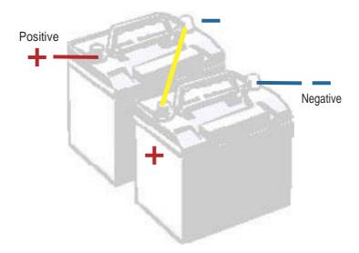
55.3 Connection of lead-acid batteries in parallel, that is positive terminal to positive terminal, negative terminal to negative terminal, will produce the same output voltage as a single battery, but the ability to supply current (capacity) will have
