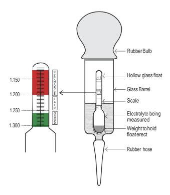
60.5 Batteries which have cells where specific gravity readings fail to rise, or respond poorly to adequate charging, should bereplaced.
