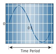
One cycle of a sinusoidal waveform is shown. This occurs in one Time Period, measured in seconds.
