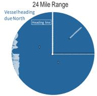
SART indication as seen on a marine radar on a bearing of 045°T. (Radar Display set to North Up)
